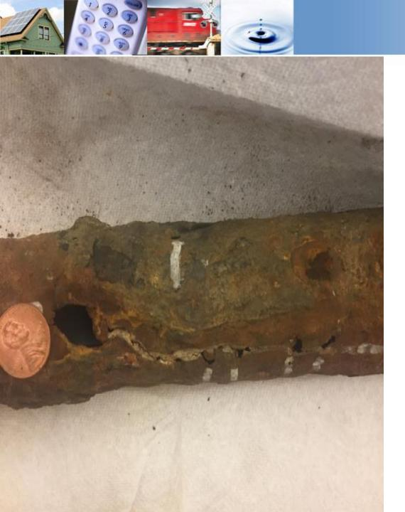
Steel pipe excavated during upgrade project exhibiting several holes
