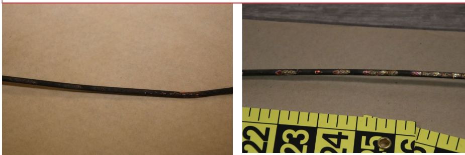
Figure 6: Damaged east conductor.
