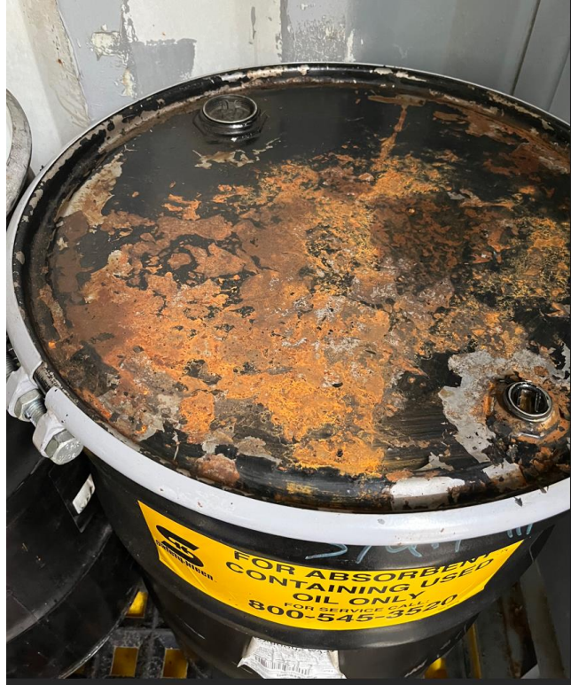
Figure 3. Waste barrel with corrosion.
