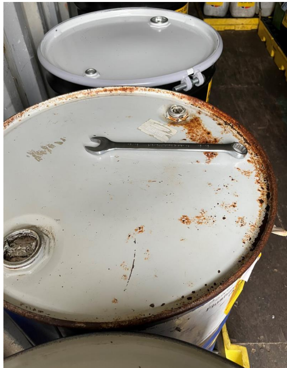
Figure 4. Second waste barrel with corrosion.
