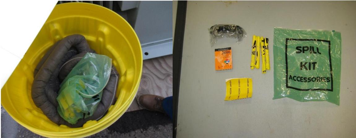
Figure 1: A spill kit and its accessories
