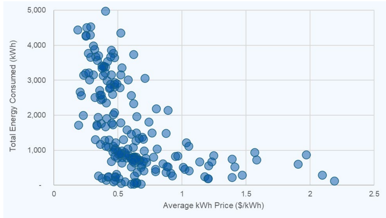
Figure 209. SDG&E PYDFP Program Monthly Energy Consumption vs. Average Energy Price for Low Consumption Billing Months (<5 MWh), PTD Sites
