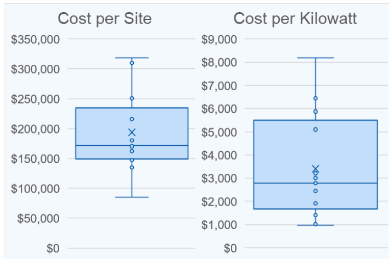
Figure 232. SDG&E Schools and Parks Pilots Average All-In Costs across 13 Closed-out PTD Sites
